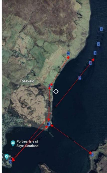
Area gas monitors to be positioned at below locations for continuous readings of H2s to the North, East, South and West from casualty location.
