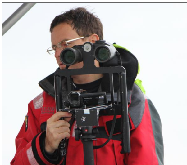
Figure 2.5: Video Range Tracking equipment
