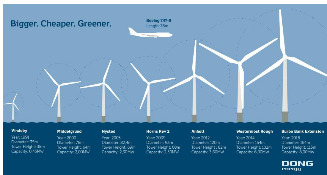
Figure 1.1: Diagrammatic representation of the progress in development of increasingly larger turbines for use in offshore wind farms. Source: humberbusiness.com ).
